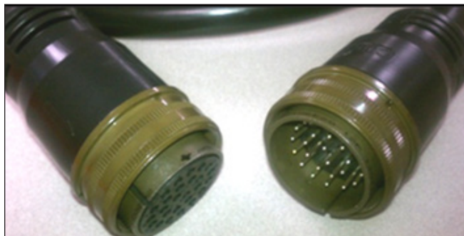
Figure 7. Cable with aluminum cable coupler ring.
